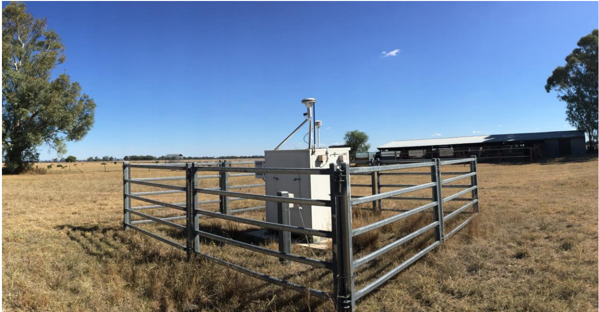
TEOM installed at Flixton property
