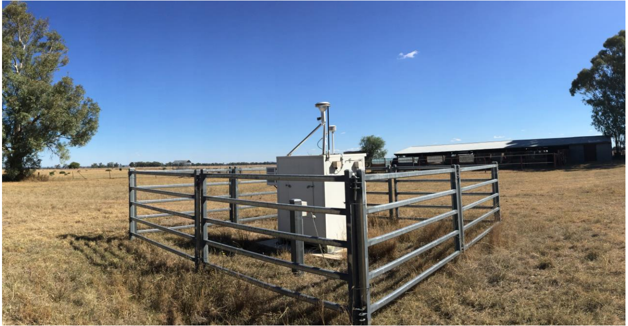
TEOM installed at Flixton property
